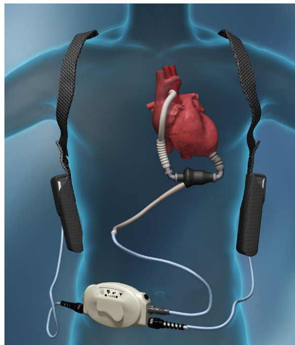
Figure 1 The HeartMate II continuous-flow left ventricular assist device receives blood from the left ventricular apex and returns it to the ascending aorta. The pump is connected with a percutaneous lead to an external controller and batteries worn by the patient.
