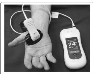
**Figure 1** Portable near infrared spectroscopy (NIRS) monitor in **use.** The probe is placed over the thenar eminence.
